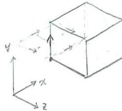
$$E_y^n = \frac{\frac{\Delta t}{\varepsilon}}{1 + \frac{\sigma \Delta t}{2\varepsilon}} \left( \frac{\partial H_x^{n-1/2}}{\partial z} - \frac{\partial H_z^{n-1/2}}{\partial x} \right) + \frac{1 - \frac{\sigma \Delta t}{2\varepsilon}}{1 + \frac{\sigma \Delta t}{2\varepsilon}} E_y^{n-1} \quad (1.44)$$
